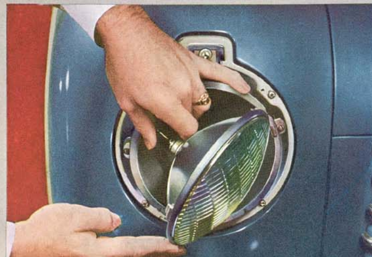
New Sealed Beam headlamps give 50% to 65% more light than the old type.
